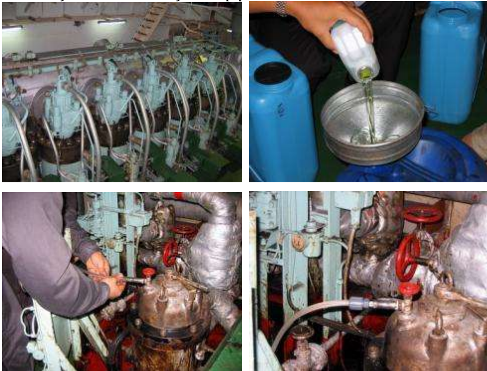
Figure 6: Addition of mXt9 TM into the fuel oil pipe line.
